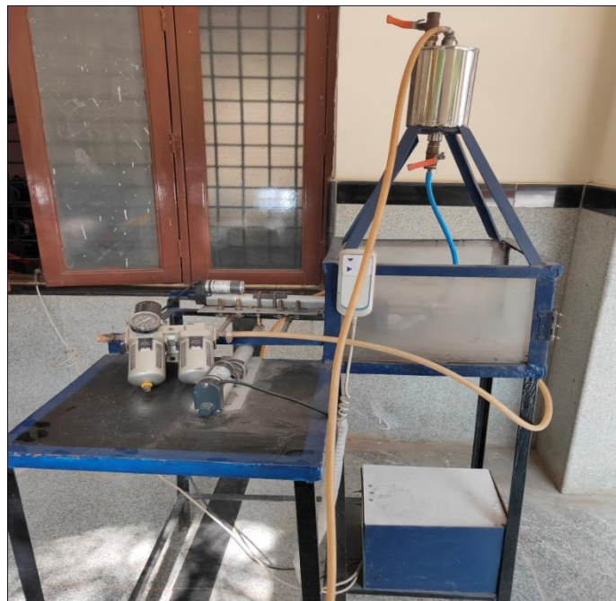
Fig. 2 Abrasive jet machining setup
